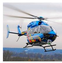
Flight tests have been completed with the electro-optical/infrared sensor turret for UH-72A Lakotas that will be operated by the US Army National Guard in Security and Support (S&S) missions. Unlike the typical EC145 law enforcement installation the L3 **Wescam MX-15** turret features a centre-line chin mount on the centre-line and has been validated during flight tests with an EC145 – the helicopter on which EADS North America's UH-72A is based.
