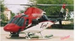
tive effect on low speed handling. For some time now it has been evident that the MRB of the 109/119 series - types well known for their high-speed cruise - suffer significant vibration when operated in a low speed orbit typical of the law enforcement mission.
