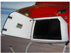
benefit from 5.5 cubic feet of increased stowing capacity per side, increased weight capacity by 100 lbs per side, a net weight increase of only 13 lb per side, easy installation and removal and yet no flight limitations
