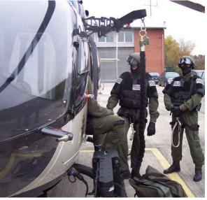
fied redundant double rope system, which supports 270kg external load, connects directly to the couplings of the EAD01 installed above the sliding door of the helicopter. The double rope system eliminates the need for ground-supported anti-rotation leashes. With an overall system weight of approx. 20kg [44 lbs], a maximum of surplus load capability is given.
