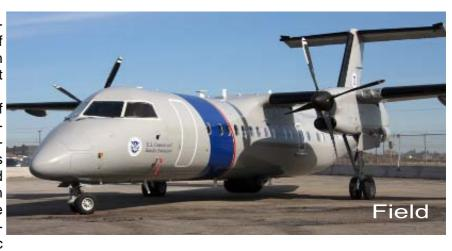
commercial airframe delivery from the manufacturer and fitted the role equipment. Features of the role fit include the Raytheon Sea Vue 20321 search radar, L3 Wescam's MX-15 EO/ IR turret and the ATK Integrated System's ISADS mission management system.
