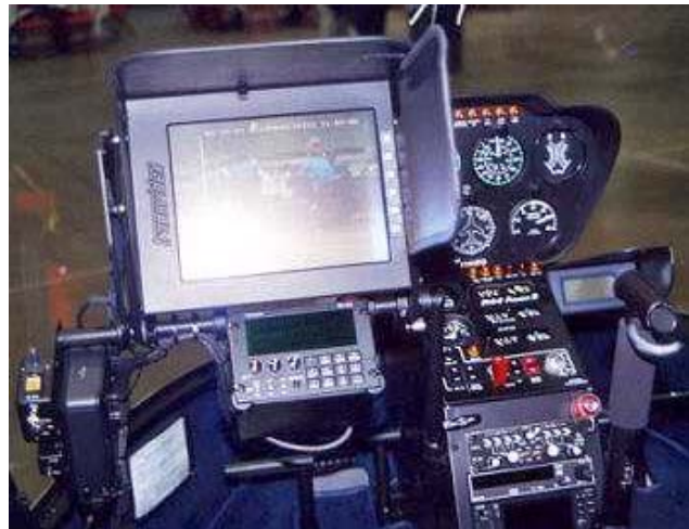
Robinson were displaying their new Raven based R44 Police and a similar Newscopter. The interior of the Police model now includes a retractable monitor that greatly enhances the direct field of vision for the observer when not using the sensor.
