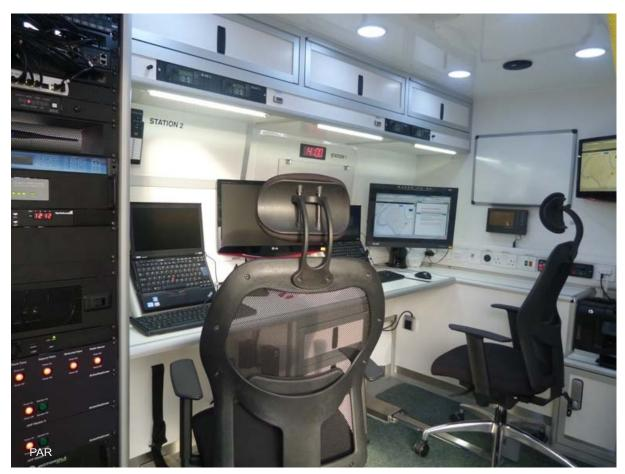
The system displayed at the show is based on a Renault van, with all network systems powered by a Honda generator, the vehicles' key communications networks provide both online and offline capabilities. The innovative vehicles are also equipped with a range of the latest communications functions ranging from 3G connectivity and WIFI routing, mobile GSM, and Airwave terminals to compliment traditional communication technology such as VHF and UHF radios.
