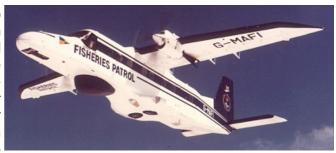
clude digital avionics and a glass cockpit and is expected to be termed the Dornier 228 New Generation.
