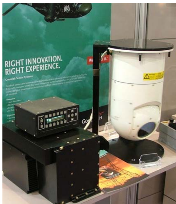
Heli-Dyne Systems were showing a range of equipment options including a universal gimbal mount for the AS350/355 series. The new unit has a bayonet quick connect gimbal mount that will accept the Wescam MX15, the FSI Star Safire series and Ultra Media LE.
