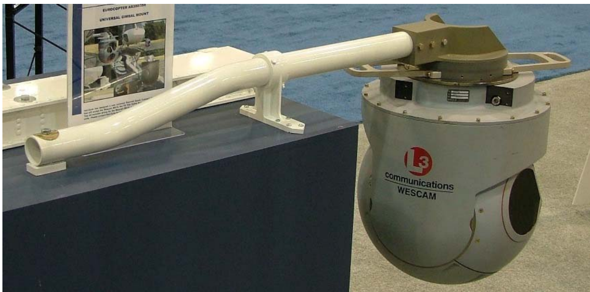
Heli-Dyne Systems were showing a range of equipment options including a universal gimbal mount for the AS350/355 series. The new unit has a bayonet quick connect gimbal mount that will accept the Wescam MX15, the FSI Star Safire series and Ultra Media LE.
