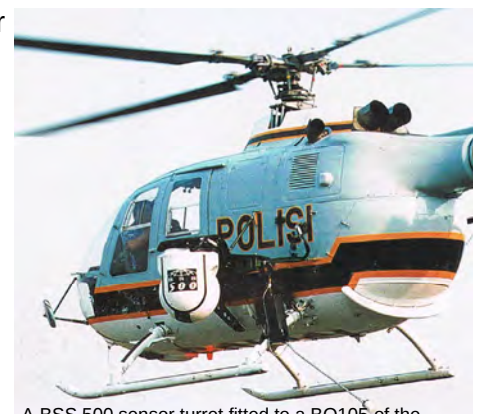
A BSS 500 sensor turret fitted to a BO105 of the Indonesian Police 'in the last century' - production is returning to West Malling.
