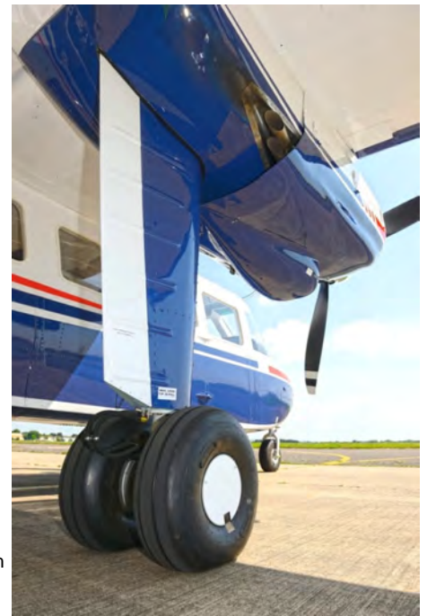
The Hartzell three-bladed scimitar shaped propeller minimises the aircraft's noise footprint through greater efficiency and reduced tip speeds. (BN)
