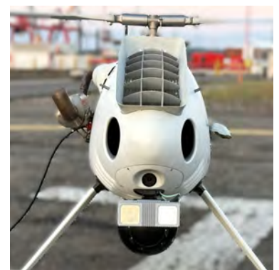
The standard Scheibel drone is fairly noisy and the NPAS model has been modified with the addition of a prominent exhaust expansion box (silencer) to meet the low noise needs of the trial. [NPAS]
