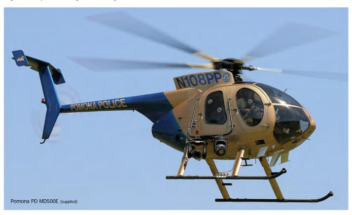
The 2008 Pomona Police Department MD-500E helicopter N108PP, on which the package is fitted, assists ground units in performing routine patrols, surveillance missions, search and rescue, counterterrorism patrols, searches, transports, speed enforcement, vehicle pursuits, and command and control for emergency incidents. The role fit utilises the usual right-side mounts below the cabin doors.
