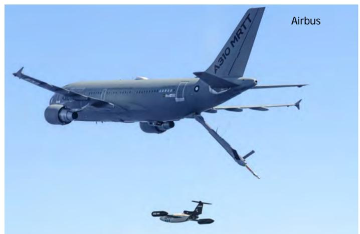
and commanded thanks to artificial intelligence and cooperative control algorithms, without human interaction. The different receivers were controlled and guided until a minimum distance of 150 feet (around 45 metres) from the A310 MRTT.
