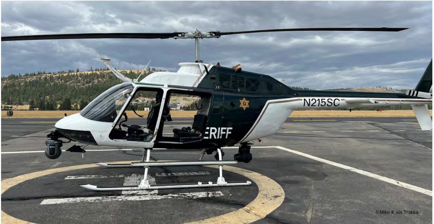
The Total Mission Solution Package consists of the #TrakkaCam TC-300 EO/IR, gyro-stabilized surveillance camera, the sophisticated multispectral #TrakkaBeam TLX Searchlight, and #TrakkaMaps TM-100 Moving Map / Video Management System installed in a 50 year old DoD surplus Bell OH58 Kiowa. A single system has been delivered.
