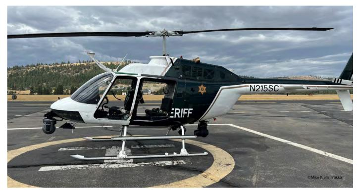
The Total Mission Solution Package consists of the #TrakkaCam TC-300 EO/IR, gyro-stabilized surveillance camera, the sophisticated multispectral #TrakkaBeam TLX Searchlight, and #TrakkaMaps TM-100 Moving Map / Video Management System installed in a 50 year old DoD surplus Bell OH58 Kiowa. A single system has been delivered.
