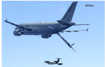
Over the waters of the Gulf of Cadiz, the control of the drone transitioned from a ground station to the A310 MRTT, autonomously guiding the DT-25 to the in-flight refueling position.
