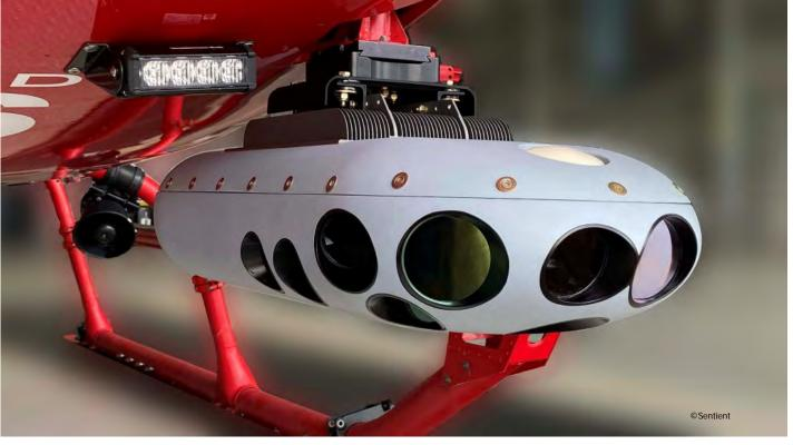
The Sentient ViDAR (Visual Detection and Ranging), the world's first Optical Radar, is a maritime wide area optical search system proven to operate up to Sea State 6. ViDAR autonomously finds objects on the surface of the ocean over vastly greater areas than traditional search methods. ViDAR operates optically so it is unaffected by white caps and other effects that impact technology such as radar.
