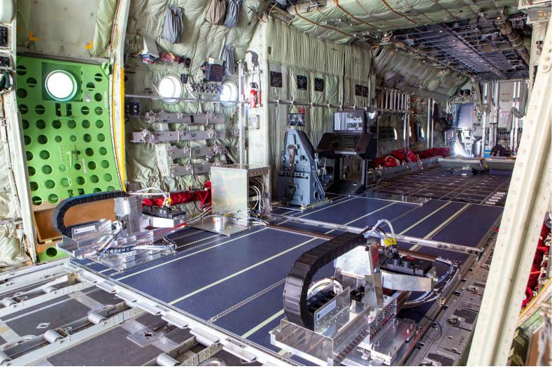
**Marshall Aerospace** based at Cambridge Airport has unveiled ARC-Radar, a modular sensor suite that allows operators of tactical transport aircraft to rapidly and temporarily outfit their fleet for intelligence, surveillance and reconnaissance (ISR) missions. ARC-Radar is the first of several products that will be rolled out within the Marshall Adaptable Role-fit Capability (ARC) family in the near future.
