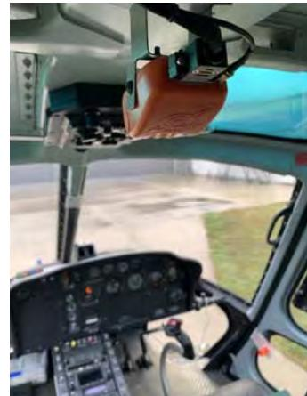
It will record speed, altitude and GPS position as well as pitch, roll and yaw data to aid the flight review process. Three audio channels capture pilot & radio, passenger and ambient cockpit audio. All data is securely stored on an SD card within a tamper proof housing, capturing 22 hours of the aircraft's latest video, audio and flight data..
