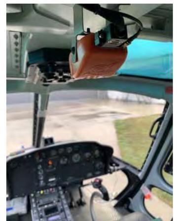
It will record speed, altitude and GPS position as well as pitch, roll and yaw data to aid the flight review process. Three audio channels capture pilot & radio, passenger and ambient cockpit audio. All data is securely stored on an SD card within a tamper proof housing, capturing 22 hours of the aircrafts latest video, audio and flight data..
