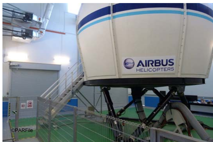
Unlike many simulators access to the cabin is via steps from below rather than a typical high level gantry.
