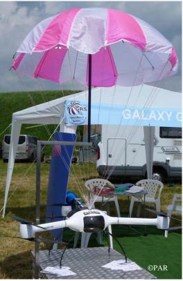
FAIL SAFE UAV At Hradev Králové an exhibitor was taking Unmanned safety to heart. This locally produced Flydeo Y6 is to include a parachute system to cover failures.
