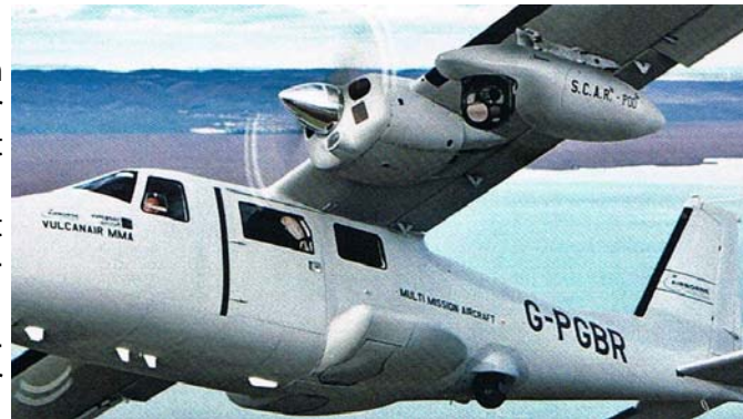
Not what it seems—the UK NPAS P68 airframe is the Photoshop demonstrator of the SCAR pod installed on a fixed wing carrier aircraft. ©Airborne Technologies
