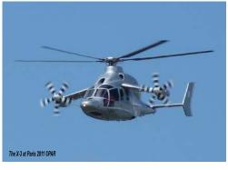
short-span fixed wings. The result is an advanced, cost effective, VTOL transportation system offering the speed of a turboprop-powered aircraft and the full flight capabilities of a helicopter.
