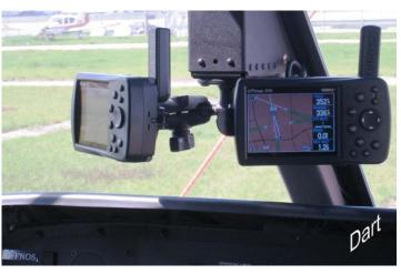
low for the simultaneous installation of two receivers that may be viewed by both pilot and co-pilot. The ball-mount system results in the receivers being adjustable to suit the varied requirements of all crew members. Once the desired position is achieved, the mount may be locked
