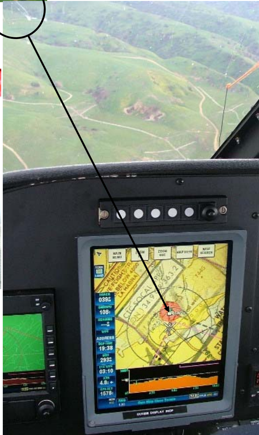
During the flight the display screen clearly highlighted a warning red ring around a near invisible obstruction in the flight path. The base of the tall slender aerials is just visible in the top left of the image but clearer highlighted above. ©PAN
