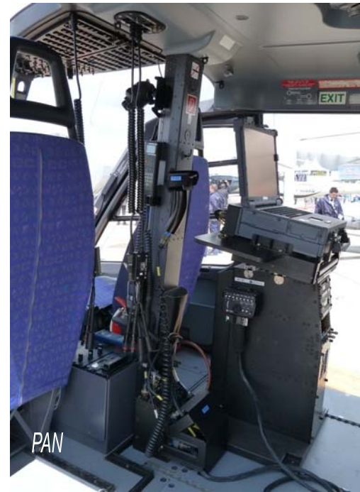
Interior rear crew station of the French Gendarmerie EC135T2 displayed by Eurocopter.
