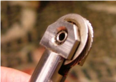
Above: Just one of the likely problems highlighted at the Goodrich maintenance workshop... unacceptable wear on the cable guide wheel of the 'crowder' tensioner.
