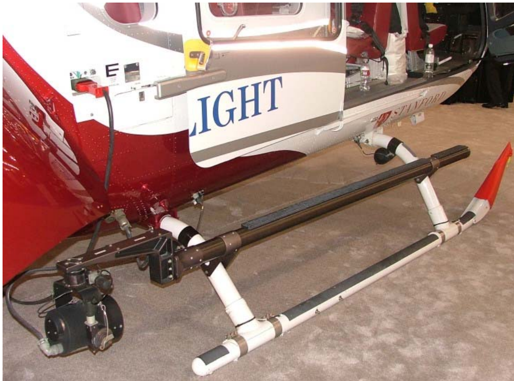
Air Methods displayed a 2006 Eurocopter EC145 N145SU c/n 9102 featuring a Meeker step carrying an SX-5 searchlight. It has been operated in the USA since 2007 and currently flies for Stanford.
