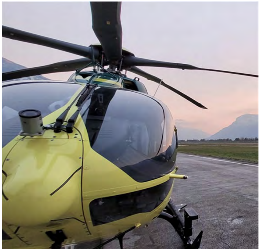
From the Global Aviation Systems GmbH Linked In Social Media account at is this illustration of the Honeywell VXP—the only manufacturer approved rotor track and balance system for the H145 D3. Honeywell by way of Diagnostic Solutions International, LLC [Global photo]
