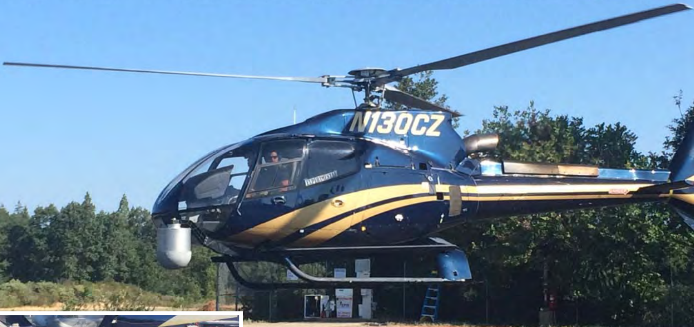
In July Cal Meeker commenced flight testing a robust new camera mount specifically for applications on the Airbus Helicopters H130 ©Meeker
