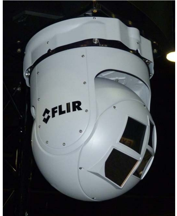
FLIR Systems Corona 350 IR systems was added to the usual line-up of gimbals by the takeover of the former PolyTech based in Sweden and has added a long sought uncooled technology system to the FLIR range.
